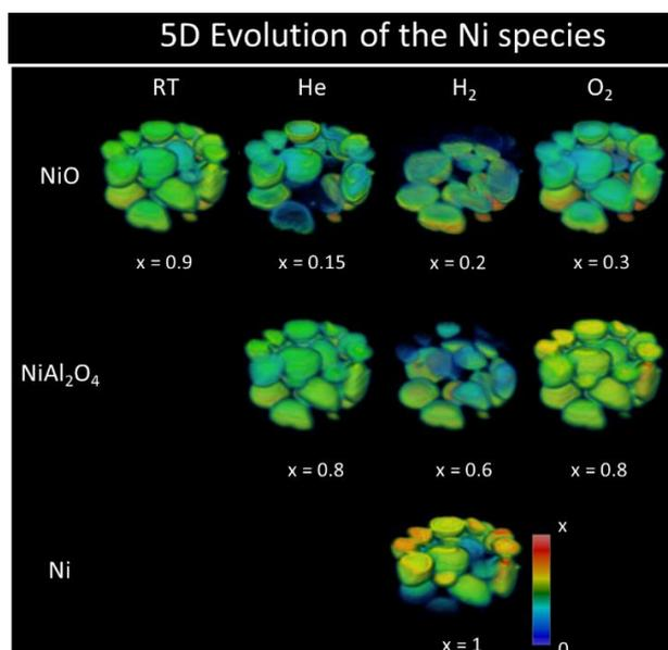
Figure 1: Phase distribution volumes of NiO, NiAl<sub>2</sub>O<sub>4</sub> and Ni as obtained from the Rietveld analysis of the 3D-XRD-CT data collected at the four different operating conditions. The values in the colorbar axes have been chosen to achieve the best possible contrast.
