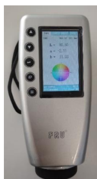
Figure 6. Portable colorimeter, the L*a*b diagram appears on the screen (left) and colorimetric measurements after 1 month of accelerated aging for pink color (right) of the real artwork.
