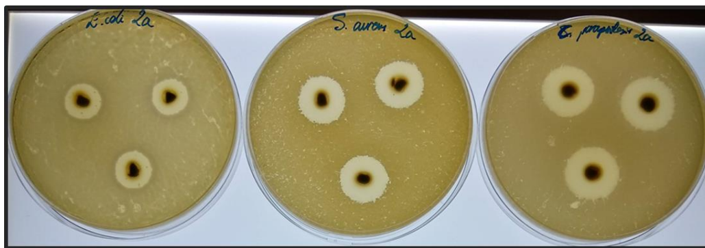
Figure. 4: Images of agar plates showing the antibacterial activity of HBPEI 0.2 Ag 0.25 Chit 0.8 film (up) and HBPEI 0.2 Ag 0.25 Chit 0.8 Gentamicin (down) against E. Coli , S. aureus and C. Parapsilosis .
