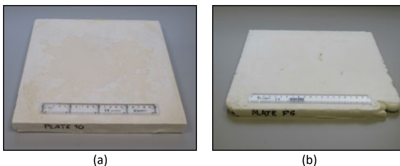
Figure 7. Rigid (a) and soft (b) PU foam specimen developed by incorporation of CDWs.
