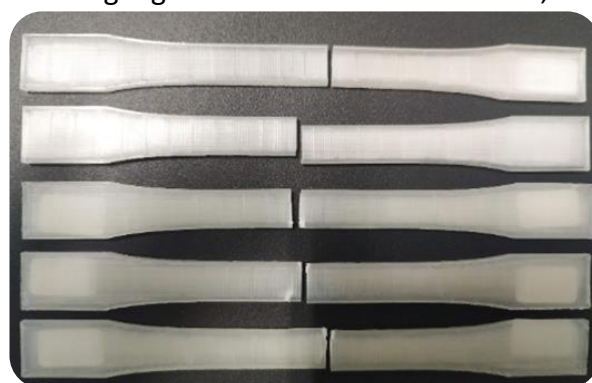
Figure 2. Tensile specimens successfully fractured in gauge section.
