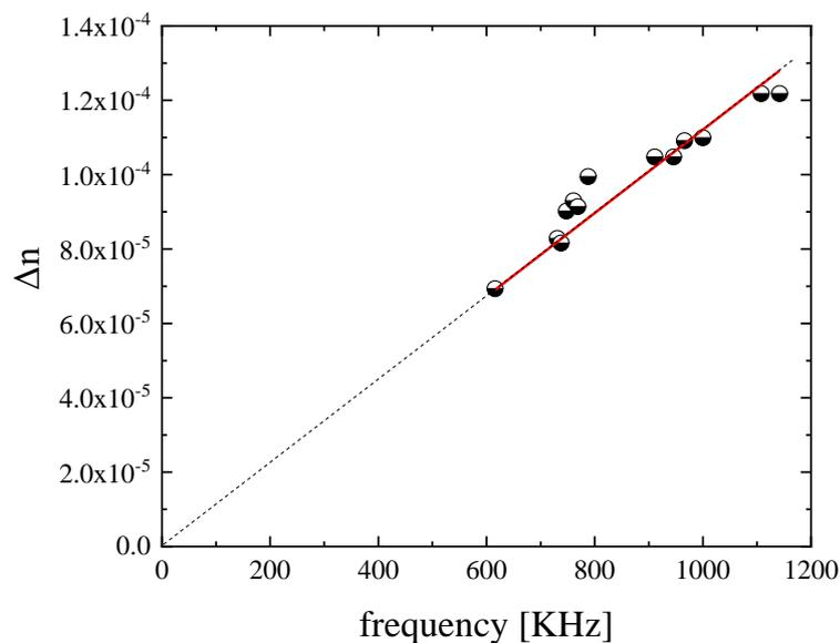
**Figure 4.** Frequency dependence of the induced birefringence for Dexa-SP dissolved in propylene glycol at 20°C. The results indicate a linear dependency between birefringence and ultrasound frequency.
