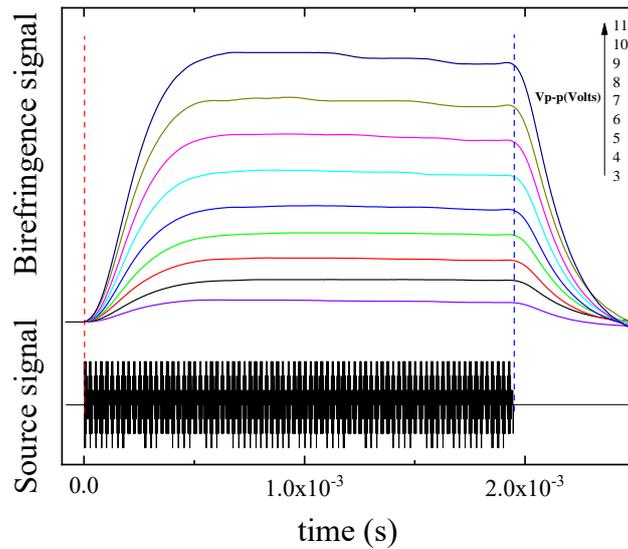
**Figure 1.** Traces of transient ultrasonically induced birefringence of 2mg dexamethasone disodium phosphate dissolved in 10ml propylene glycol at 20°C for all applied voltage to the transducer. The frequency of the ultrasound waves applied to the liquid sample was 770 KHz. The applied ultrasonic pulse is also shown for comparison.
