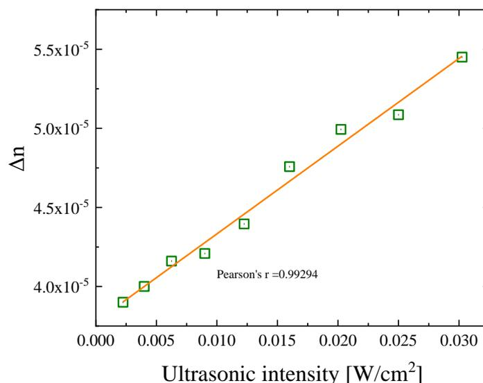
**Figure 2.** Induced birefringence as a function of ultrasonic intensity of DEX-SP dissolved in propylene glycol at 20°C. The value of Pearson's  $R=0.99294$  indicates an almost perfect linear dependency between birefringence and ultrasonic intensity. The frequency of the ultrasound waves applied to the liquid sample was 770 KHz.
