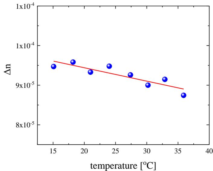
**Figure 3.** Temperature dependence of the birefringence for Dexa-SP dissolved in propylene glycol at 20°C. The results indicate a linear dependency between birefringence and temperature.
