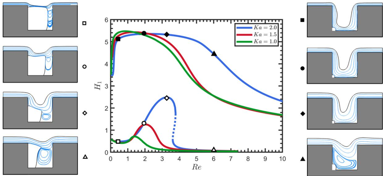
**Figure 2** Map of the steady-state solutions in terms of the wetting distance  $H_1^*/\sqrt{\frac{\rho^* g^*}{\sigma^*}}$  for  $Ka = 1, 1.5, 2$ ,  $\theta = 60^\circ$  and  $\alpha = 90^\circ$  for  $d = D^*/\sqrt{\rho^* g^*/\sigma^*} = 6$  and  $w = W^*/\sqrt{\rho^* g^*/\sigma^*} = 6$ . The symbols in the solution families correspond to one of the flow patterns around the figure.
