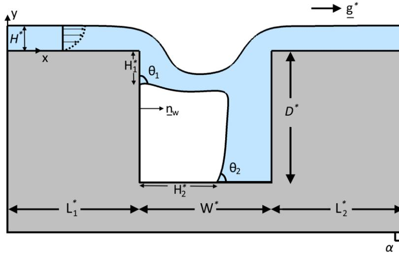
**Figure 1** Cross section of the film flowing over a rectangle trench with air inclusion at the upstream corner. The geometric parameters, the orientation of the substrate, the unit vector of the wall and the contact points angles are indicated, while the film thickness at the entrance is  $H^*$ .
