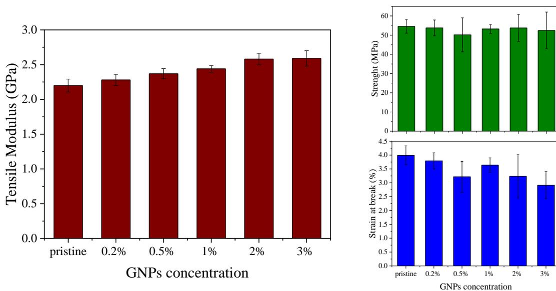
**Figure 2.** Tensile properties of pristine and different concentrations GNP/epoxy nanocomposites films.
