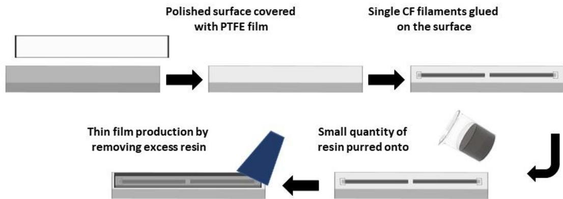
**Figure 1.** Model composite fabrication
