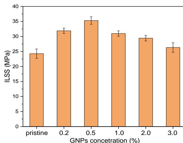
**Figure 4.** Interlaminar shear strength values of pristine and different concentrations GNP/epoxy nanocomposites films.
