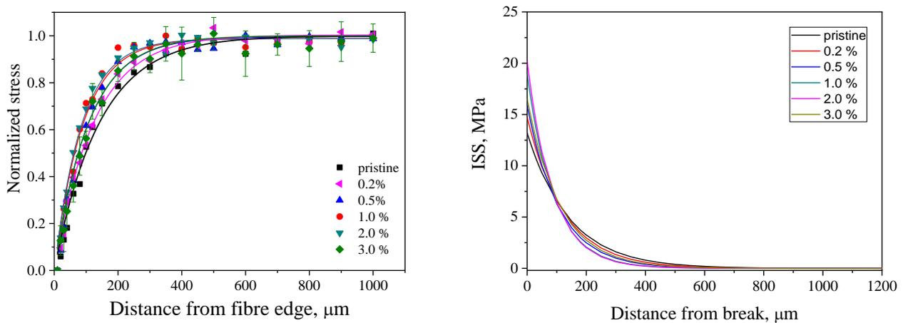
**Figure 3.** Normalized axial stress (left) & ISS (right) versus the distance from the discontinuity of CF embedded in the epoxy resin for different GNP concentrations.
